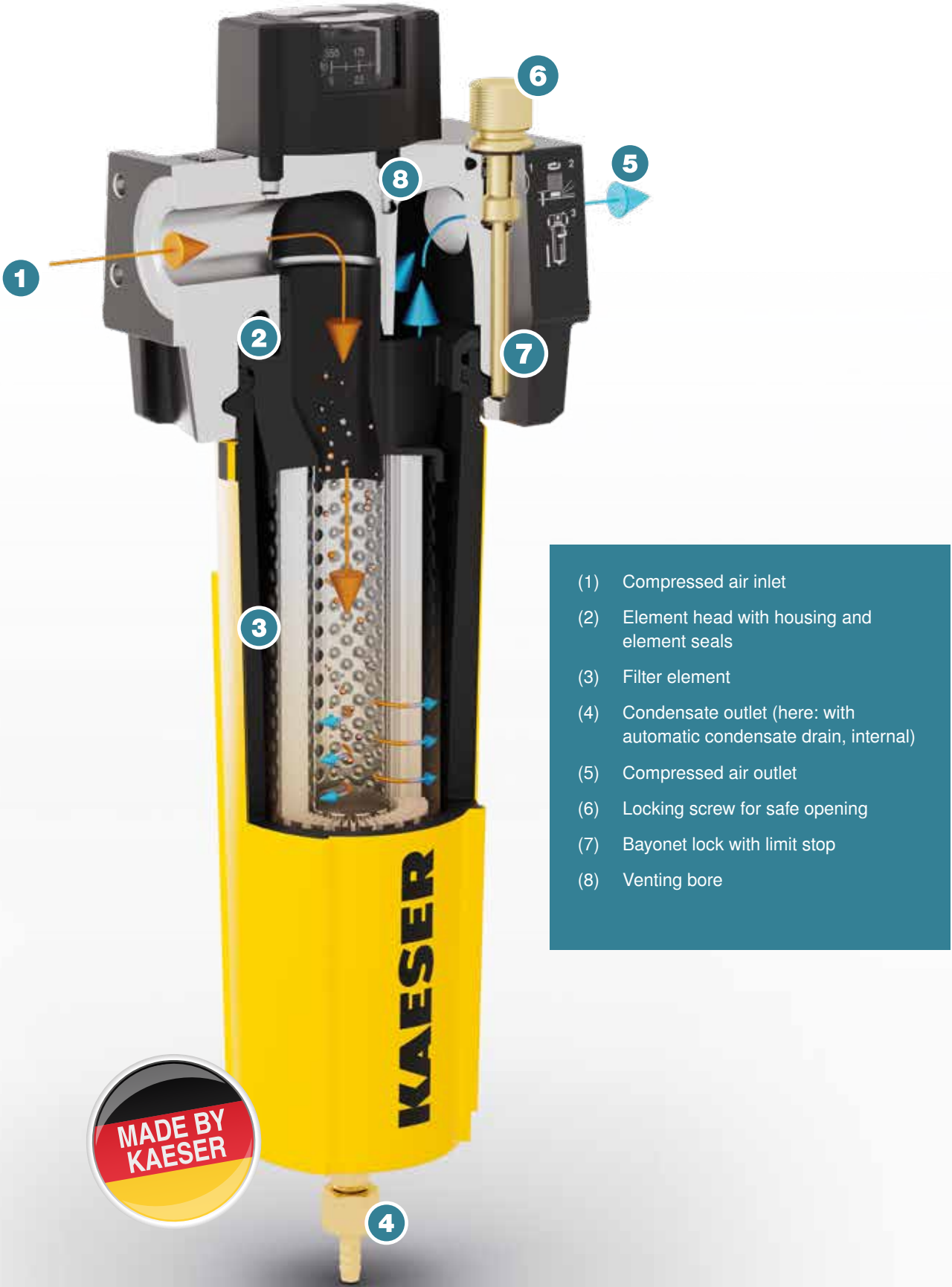
Image: Functional diagram, coalescence filter
